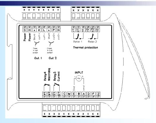
mV input from: terminal A (+), terminal E (-) external shunt
